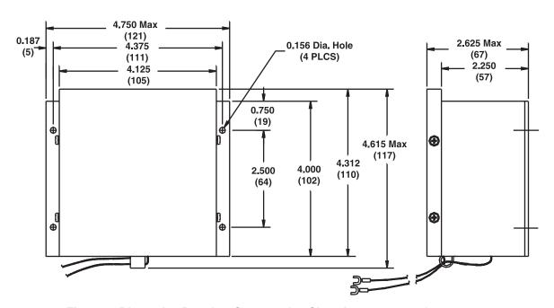
Figure 7 - Dimension Drawing, Suppression Chassis 9261500100/101
