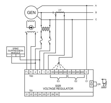
Figure 3 - Typical Interconnection Diagram
