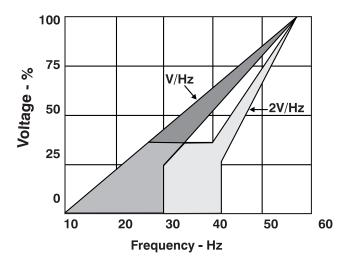
Figure 2 - 60 Hz Frequency Compensation
