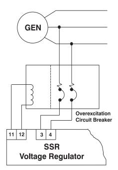
Figure 4 - Typical Overexcitation Circuit Breaker Interconnection
