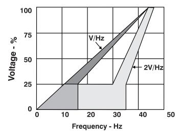
Figure 1 - 50 Hz Frequency Compensation
