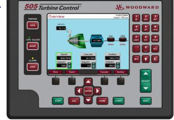
required to control steam plant parameters like turbine speed, turbine load, turbine inlet header pressure, exhaust header pressure, or tie-line power.
